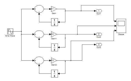
2 Select the Sum, Gain, and Unit Delay blocks and create an atomic subsystem with inputs U, U1, and U2 and outputs Y, Y1, and Y2. Rename the Subsystem block as SimpleSubsytem. When you are finished, the top model and atomic subsystem model look like the following model:
