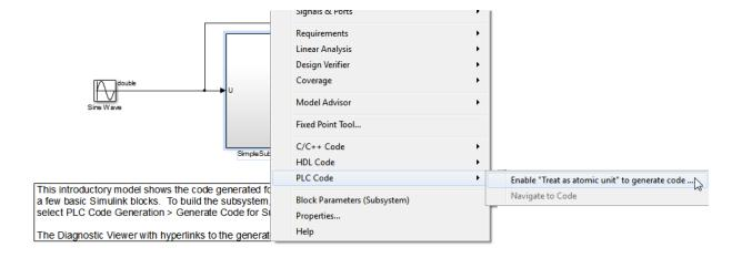
This command opens the block parameter dialog box so that you can select the **Treat** as atomic unit check box.
