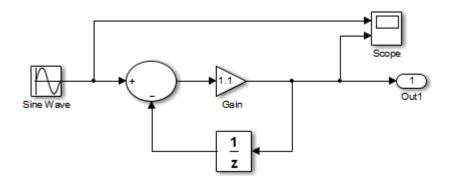
2 Configure the model to use the fixed-step discrete solver. Select Simulation > Model Configuration Parameters and in the Solver pane, set Type to Fixed-step and Solver to discrete (no continuous states).
