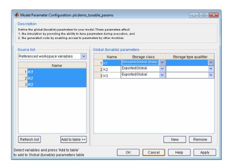
By default, this dialog box sets all parameters to the SimulinkGlobal (Auto) storage class. This setting generates code with the tunable parameters set at the local level. In this case, these parameters appear at the function block level in each function block that uses the parameter.
